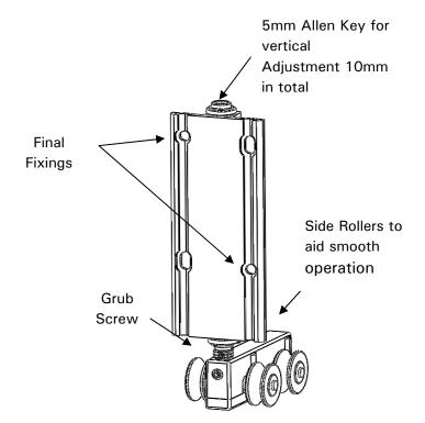
The single leaf roller is screwed directly in to the door sash euro-groove (top & bottom rollers) the rollers themselves have 10mm of adjustment (+ &- 5mm).
